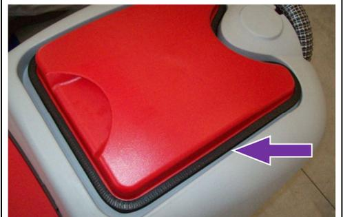
4. Check the connections and sealing of the vacuum hoses and squeegee hose.
