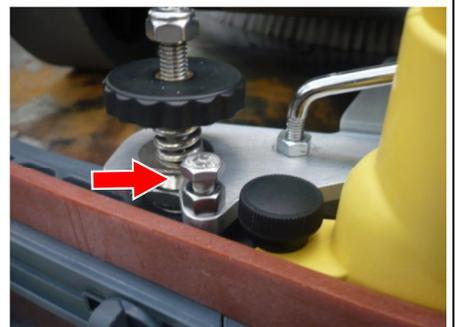
4. Check that you have an even inclination of the blade for all its length. The inclination has to be between 30° and 45°.
