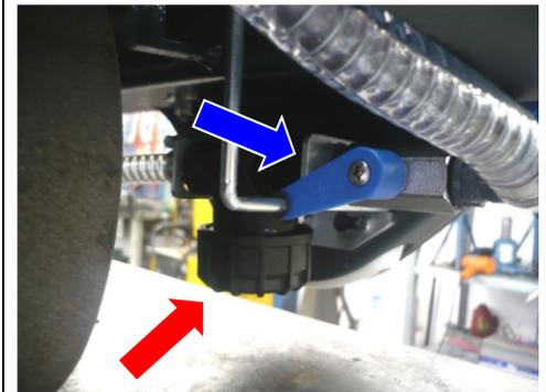
6. Check the **detergent tank drainage tap**.
