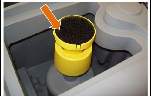
3. Check the seal between the **vacuum head** and the recovery tank.
