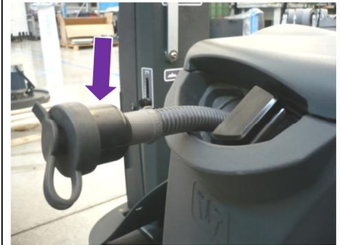
2. Check the cleanliness and sealing of the **solution filter**.
