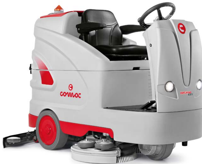
OPTIMA 85/100 B Version with disc brushes suitable for even floors with no solid debris
