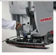
Built in battery charger kit on request, suitable for traditional and gel batteries
