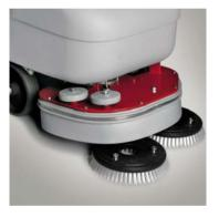
The scrubbing heads with two contrarotating brushes of Abila 42/52 and the single-brush of Abila 17/20 have adjustable inclination for better forward movement of the machine. In addition, they can be lifted by a pedal for easier machine transfer and brush maintenance procedures. In the Bt versions the two brushes are completely horizontal which improves washing power
